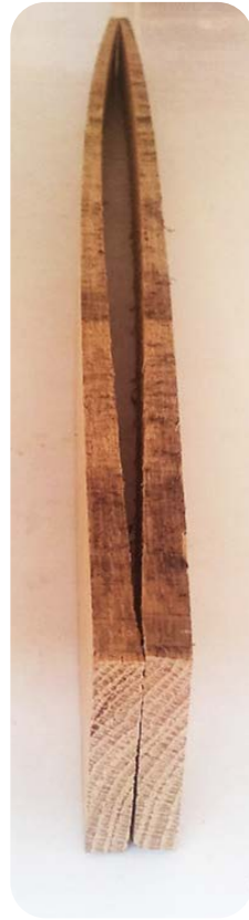
Two-inch oak board showing excessive bow after ripping due to the presence of case-hardening.
